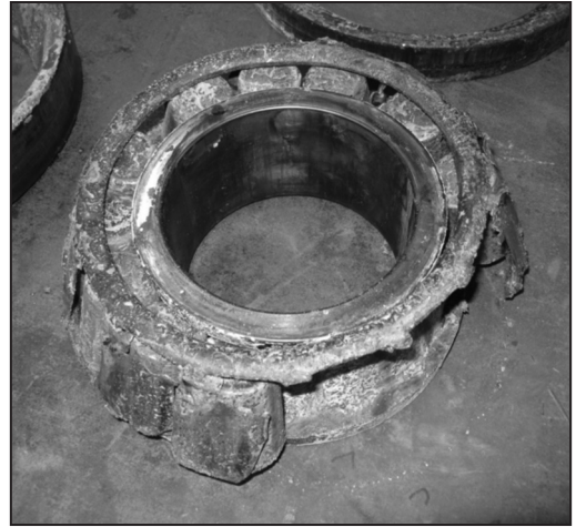
Figure 2. Failed cutter bearing
