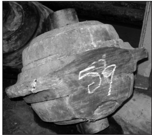
Figure 3. Non-rotating cutter damage
