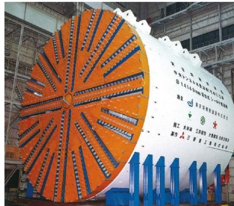
Figs. 4 and 5 Modern slurry TBMs with small cutterhead opening ratios
