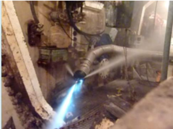
Fig16. Jet Snake Courtesy of OCRobotics
