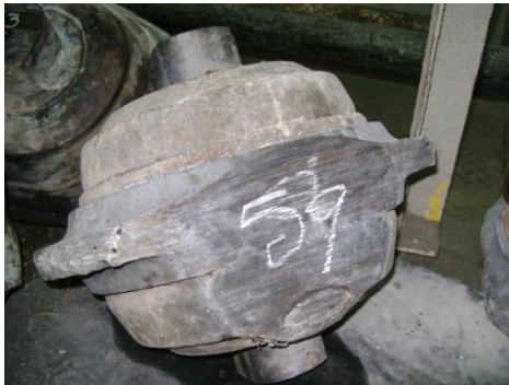
Fig 13. Non-Rotating Cutter Damage
