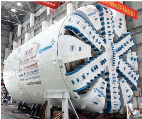
Figs. 4 and 5 Modern slurry TBMs with small cutterhead opening ratios
