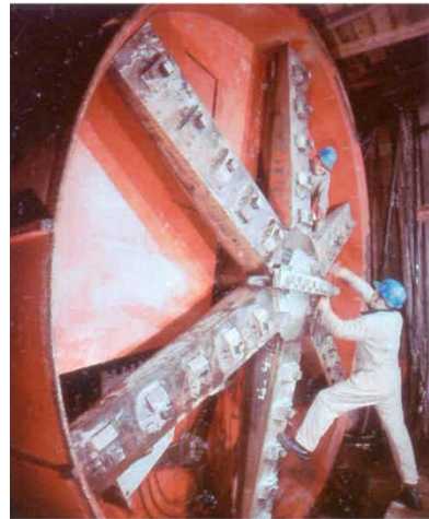
Fig 3. 1974 4.5m Hydroshield Courtesy of Wayss & Freytag
