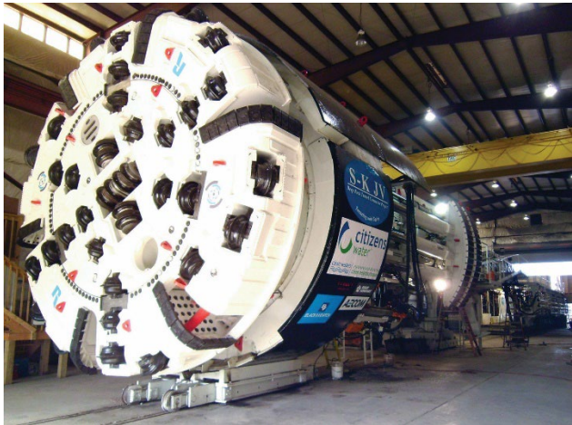
Figure 3. The DigIndyTBM, originally built in 1980, was fitted with a new back-loading cutterhead and VFD motors, among other upgrades.
